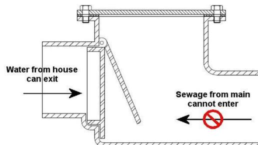
have had backwater valves installed. However, like all mechanical devices, backwater valves need periodic inspection and maintenance. Materials in household waste may get caught on the valve and block its operation. If a "sewer snake" has been used to clear a clogged drain line, the sewer snake could break the flapper valve or knock it off its hinge so it cannot operate. Homeowners should check their backwater valves about once a year to ensure they are in proper operating condition.
