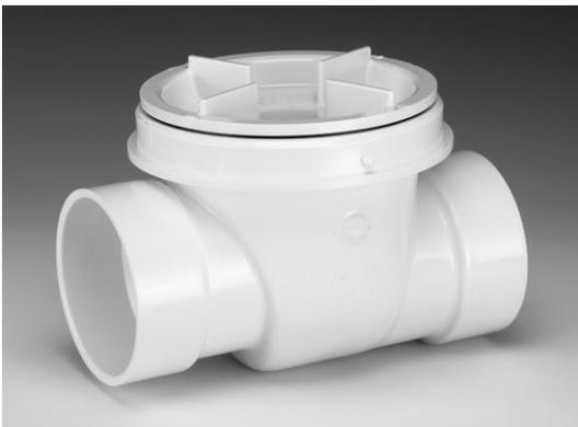
A backwater valve is a "flapper valve" that has a flat flange hinged at the top. When you use water in your house, wastewater from your household drains push the flapper open and allow wastewater to flow to the City's sewer main. But if the City's main becomes plugged causing sewage to back up, the sewage flowing toward your house pushes the flapper closed so sewage cannot enter.
